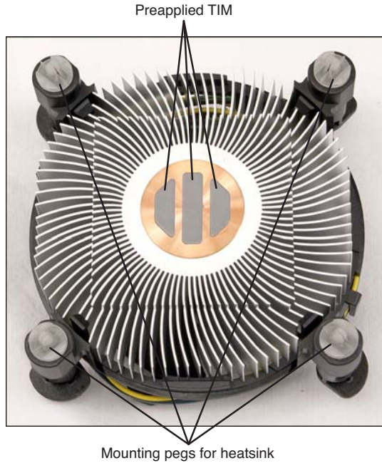
FIGURE 18.9 An Intel heatsink with preapplied TIM.
