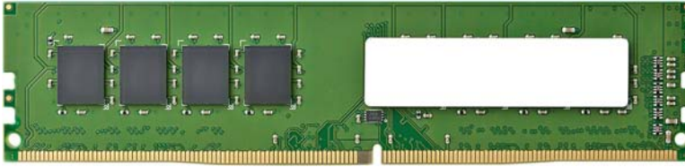
FIGURE 6.5 A typical 8GB DDR4 module without heat spreaders.
