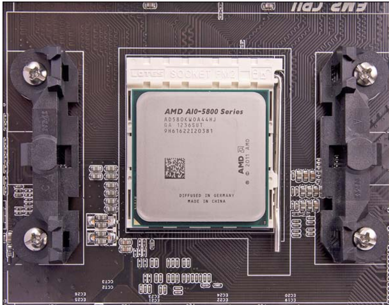
FIGURE 18.8 An AMD A10 5800K processor after being installed in an FM2 socket.
