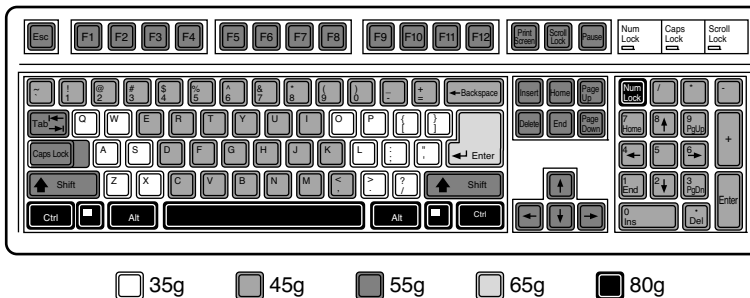
FIGURE 14.5 Force levels used on KeyTronicEMS keyboards with Ergo Technology.
