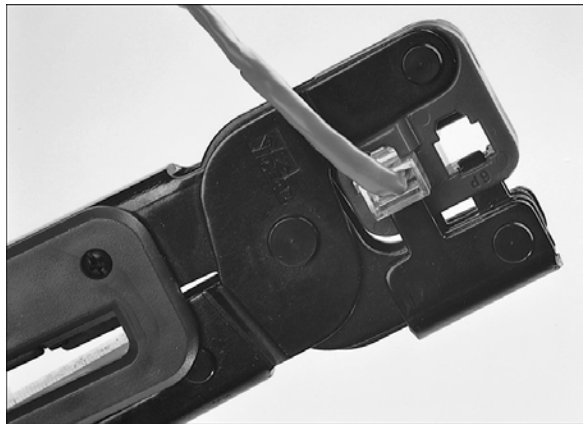
FIGURE 16.13 Firmly squeeze the crimping tool to attach the connector to the cable.
