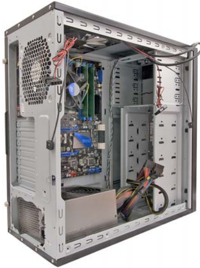
FIGURE 18.23 Installing the power supply into the chassis.
