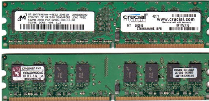
FIGURE 6.17 Markings on a 512MB DDR2 module (top) from Crucial Technology compared to markings on a 2GB (bottom) DDR2 memory module from Kingston Technology.
