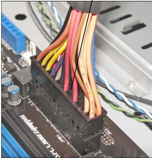
FIGURE 18.25 Attaching a 24-pin ATX motherboard power connector.
