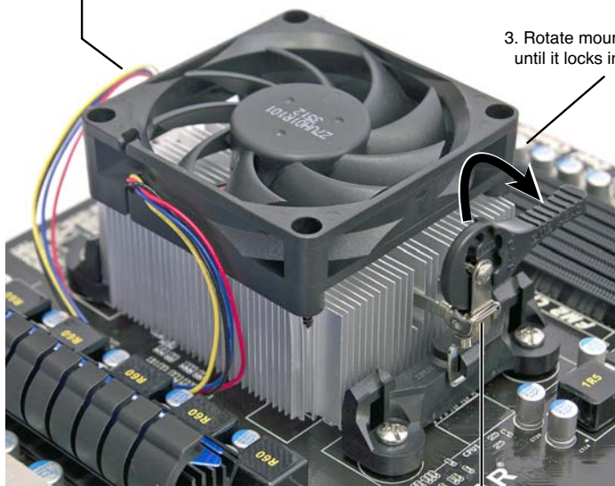
FIGURE 18.12 An AMD heatsink that clips to the frame around the processor socket.
