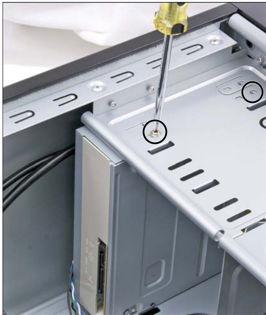
FIGURE 18.30 Secure the drive to the chassis or drive cage using four screws, two on each side of the drive.
