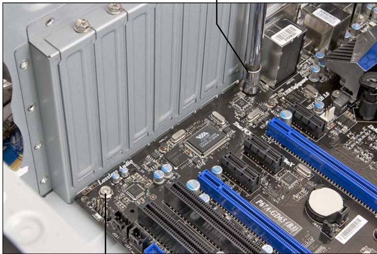
FIGURE 18.21 Installing the screws that hold the motherboard to the chassis.
