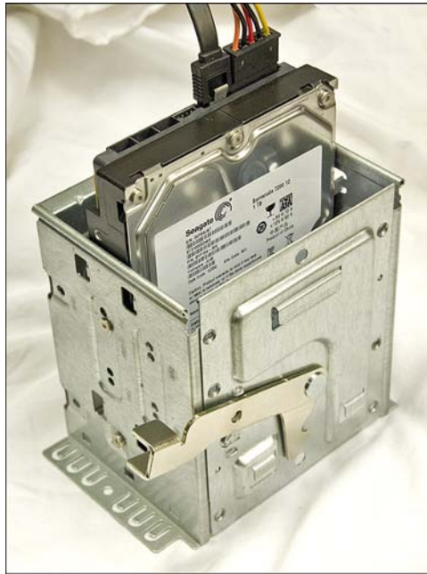
FIGURE 18.29 A hard disk drive mounted in a removable drive cage.
