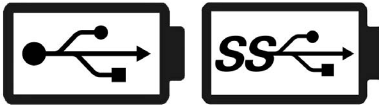
FIGURE 13.16 Typical identification marks for USB 2.0 (left) and USB 3.0/3.1 (right) Power Delivery cables.
